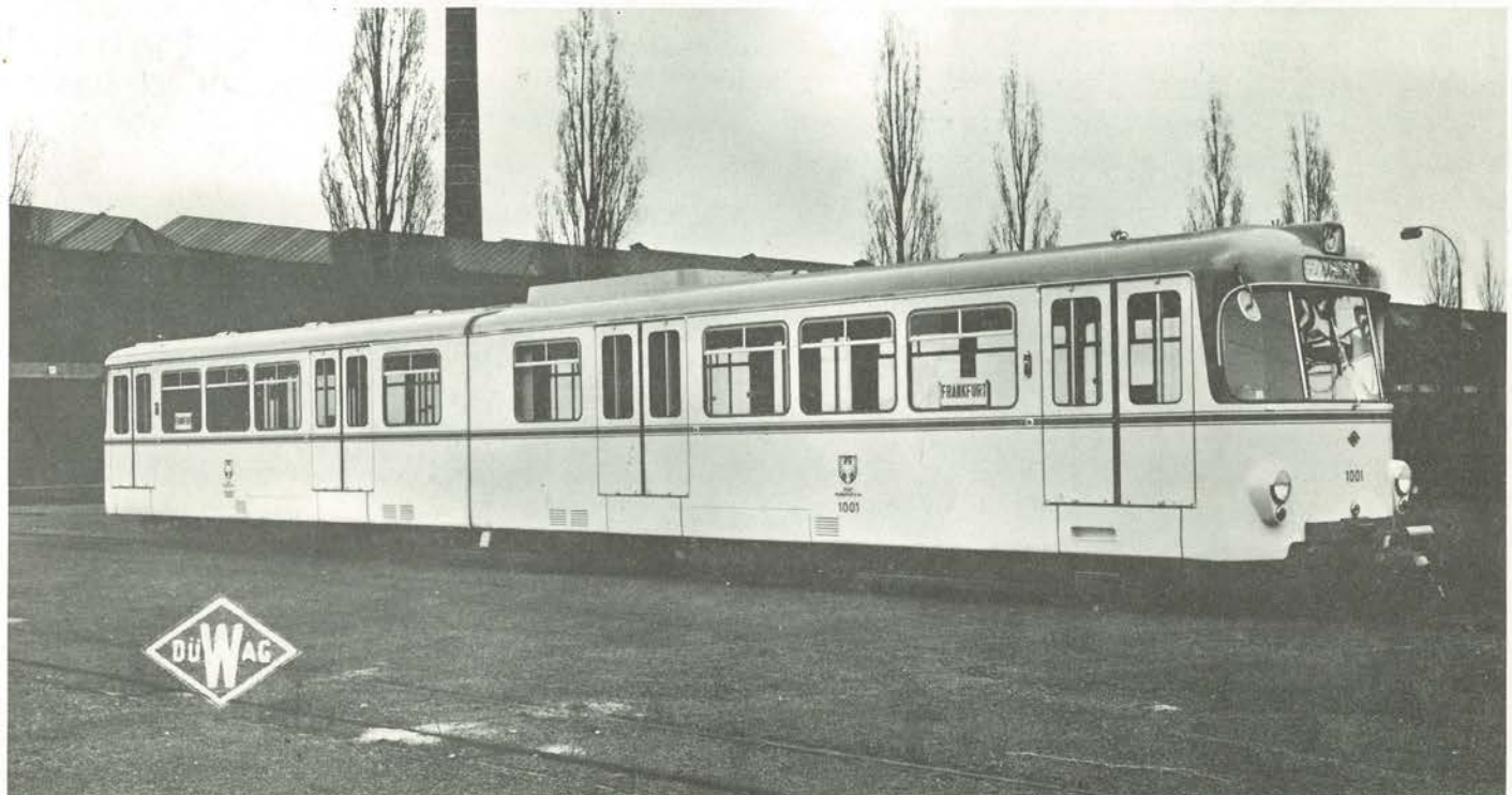
MODERN SUBWAY CAR for use on light-volume rapid transit system now under construction in Frankfurt-am-Main, Germany. Roll-up steps enable this car to load passengers from high (car-floor level) platforms in the downtown subway, and from low platforms on surface sections of the lines. photo by DuWag.
