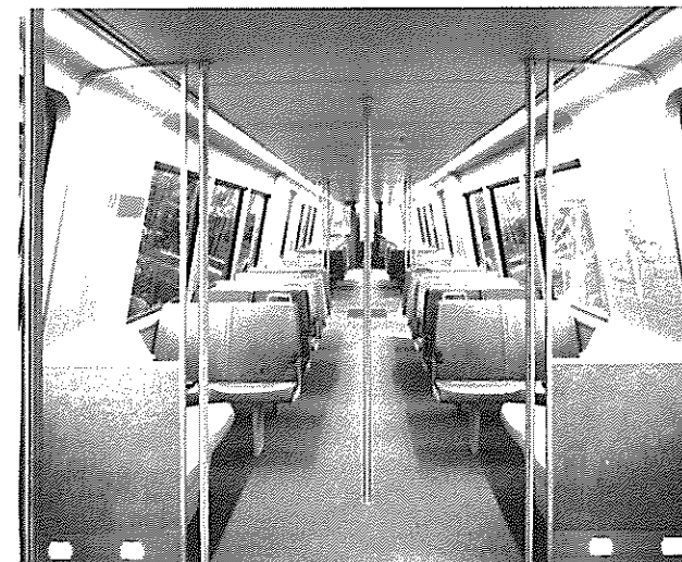
The interior of the air-conditioned Metro transit car is outfitted with sculptured bucket seats arranged two-by-two to allow each passenger generous space. The seating capacity is 82 plus 79 standees. Hand grips on the seats will eliminate strap hanging and large tinted windows provide a panoramic view without harsh glare.
