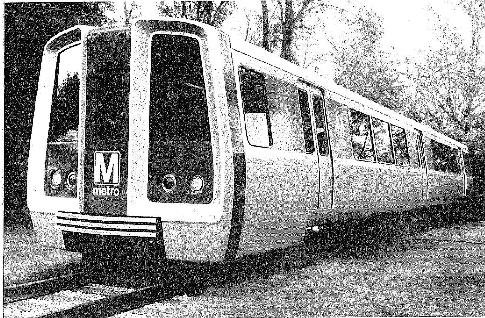
The prototype of the Metro transit car has a sculptured, contemporary design featuring a polished metal exterior and tinted panoramic windows. Passengers will enter the vehicle through three, 50-inch-wide double doors on each side. When the Metro is completed, more than 800 cars will carry millions of commuters per year in air-conditioned comfort at speeds up to 75 miles per hour. Metro will offer two-minute rush-hour service on main routes with maximum 8-car trains.
