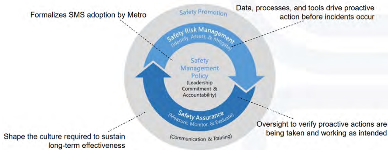
Figure 15: Components of a Safety Management System
