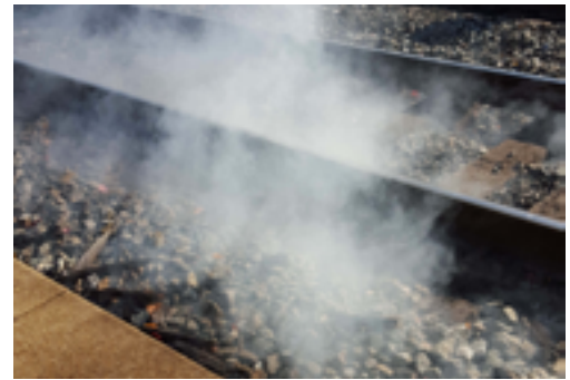
Smoke was expected to come up concentrated between the tracks but instead appeared dispersed along the length of Track 3, suggesting a blocked or collapsed pipe.
