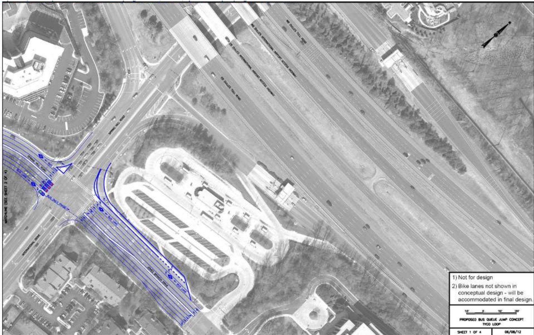
Figure A 12: Proposed Queue Jumps and Exclusive Bus Lanes –Spring Hill Road at International Drive
