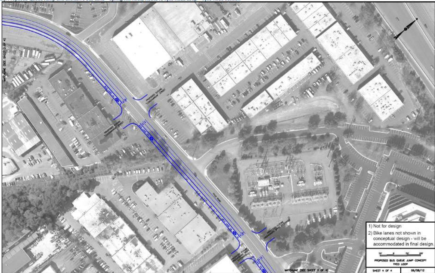
Figure A 15: Proposed Queue Jumps and Exclusive Bus Lanes – Driveways along Tyco Road
