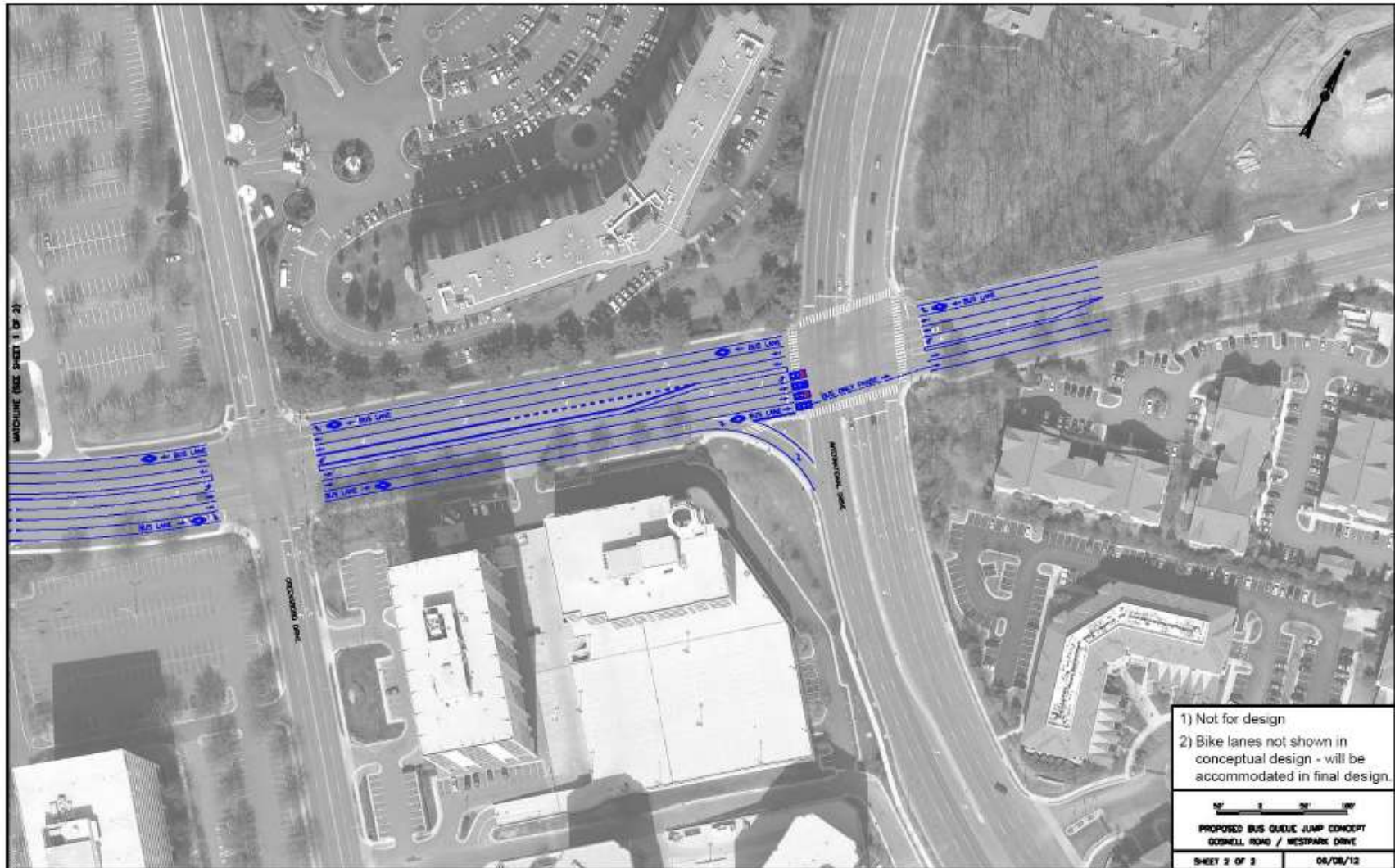
Figure A 11: Proposed Queue Jumps and Exclusive Bus Lanes –Westpark Drive at Greensboro Drive and at International Drive
