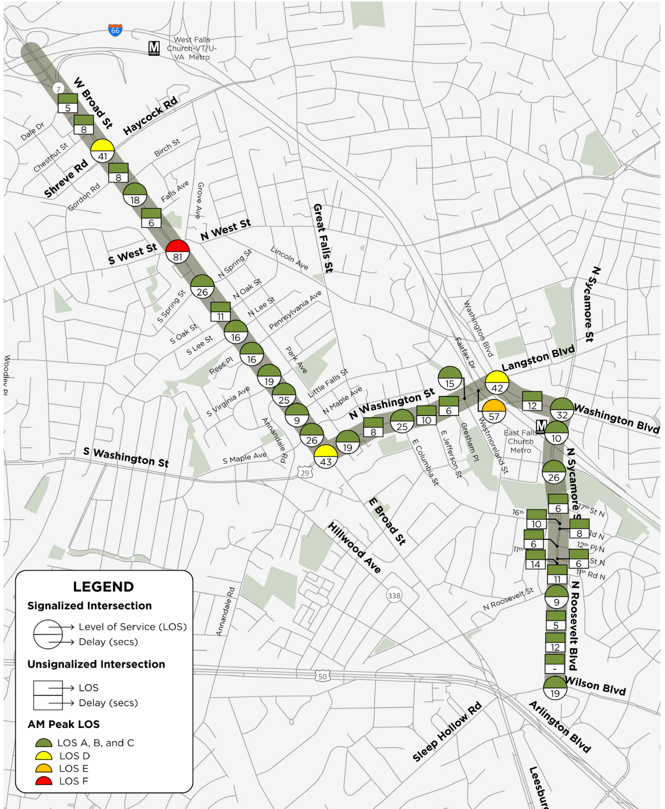
Figure 5-5: Build Scenario 1 Intersection LOS and Vehicle Delay for the Morning Peak Hour
